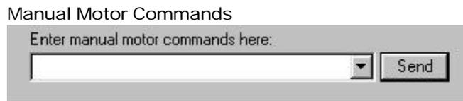
The manual motor command entry area is at the bottom of the motor control window. Here, you may type in the microcontroller commands to directly change the motor settings and movement.
