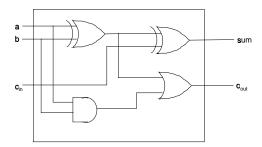
We don't need to worry about the internals but just need to realize that the circuit has three inputs,  $a_i, b_i, c_i$  and produces  $s_i$  and  $c_{i+1}$ . To produce a two bit adder we can simply cascade a pair of them together. The only trick is that the first sum doesn't have a signal for the carry input of the first full adder. But this is no problem- since there is no initial carry in we can just set that to 0. The implementation is then:
