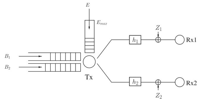
**Fig. 2.** The two-user fading broadcast channel with an energy harvesting transmitter.
