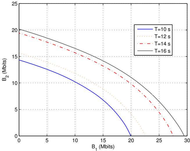
Fig. 8. The maximum departure region for the parallel broadcast channel under the given energy arrivals for various  $T$ .
