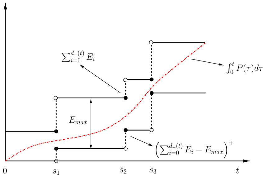
Fig. 5. Energy causality constraint and no-energy-overflow constraint are depicted as cumulative energy curves and the power consumption curve of a transmission policy that simultaneously satisfies these two constraints by lying in between these two curves.
