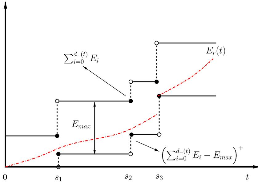
Fig. 4. The total removed energy curve  $E_r(t)$ . The jump at  $s_3$  represents an energy overflow because of the finite-capacity battery.
