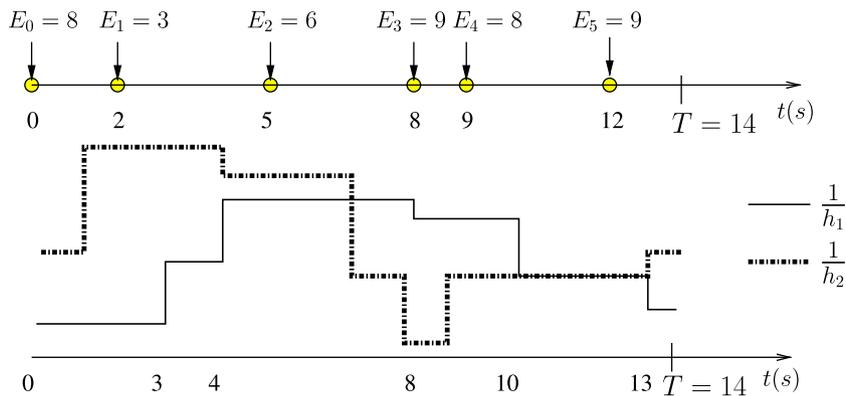
Fig. 9. The energy and fading profiles for the fading broadcast channel.
