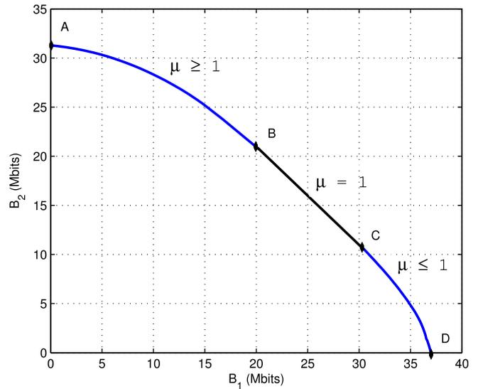
Fig. 10. The maximum departure region for the fading broadcast channel under the given energy arrival and fading profiles at  $T = 14$  s.
