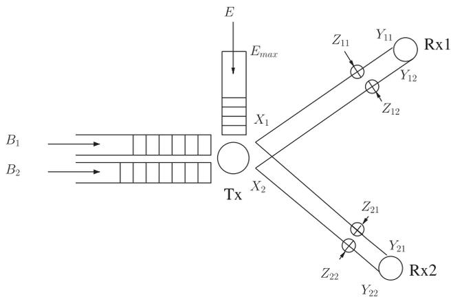
**Fig. 1.** The two-user parallel broadcast channel with an energy harvesting transmitter.
