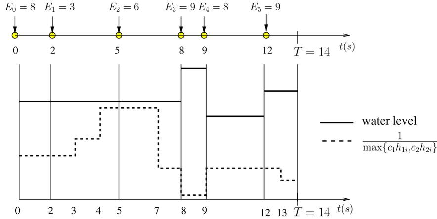
Fig. 11. The sum throughput optimal policy obtained by directional water-filling.
