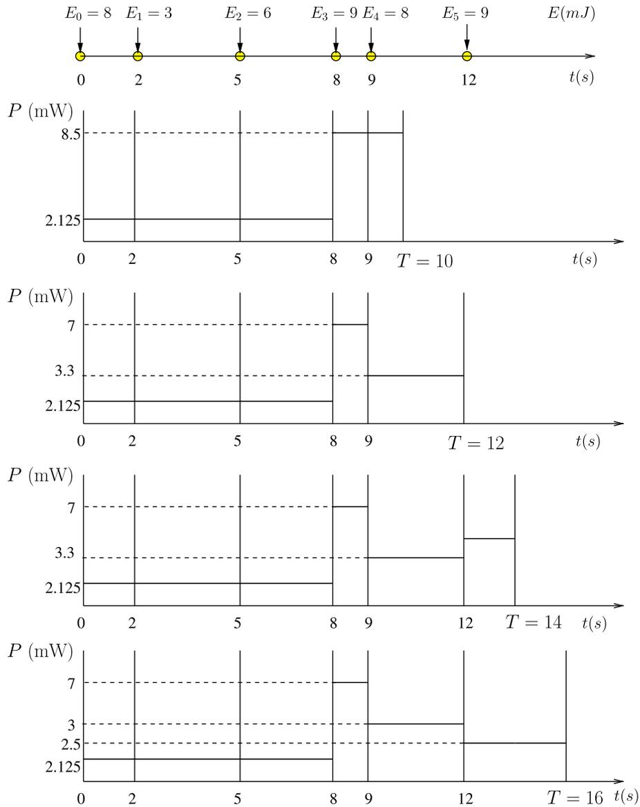
Fig. 7. Energy arrivals occur at [2, 5, 8, 9, 12] s with amounts [3, 6, 9, 8, 9] mJ and the initial energy in the battery at time zero  $E_0 = 8$  mJ. The optimal total power sequence for  $T = 10$  s,  $T = 12$  s,  $T = 14$  s and  $T = 16$  s.
