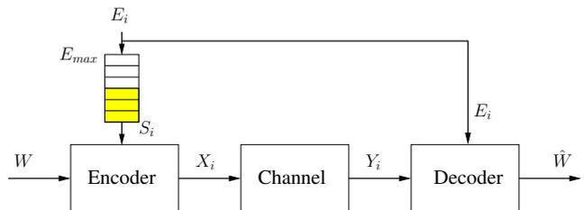
Fig. 1. The channel with an energy harvesting transmitter with a finite-sized battery. The energy arrival information is available at both sides.
