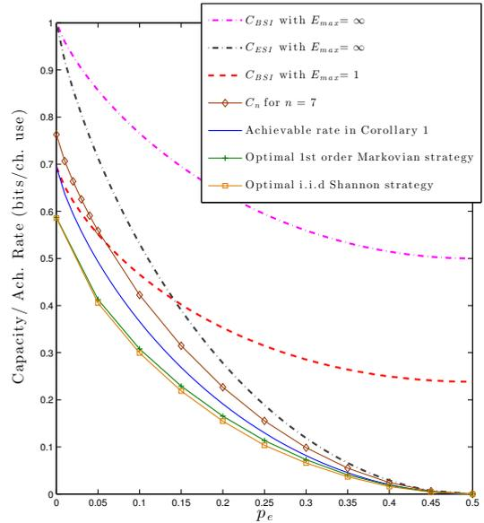
Fig. 3. The capacities with energy arrival and battery side information at the receiver side and achievable rates with side information only at the transmitter in a BSC( $p_e$ ). The plot is with respect to the channel crossover probability  $p_e$  for  $P[E_i = 0] = 0.5 = P[E_i = 1]$ .
