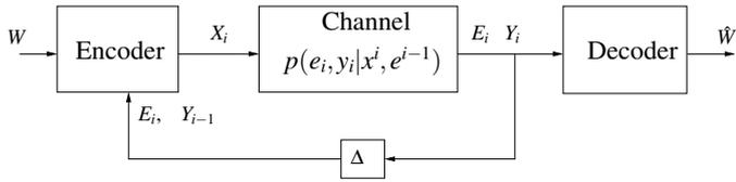
Fig. 2. Virtual channel model with feedback. Presence of the channel output feedback  $Y$  does not affect the capacity.
