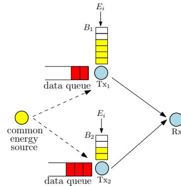
Fig. 1. System model: an energy harvesting multiple access channel model.
