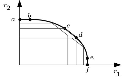
Fig. 2. Capacity region of a multiple access channel.
