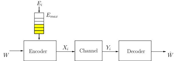
Fig. 1. The binary energy harvesting channel (BEHC) model.
