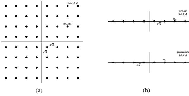
Fig. 1. (a) A 64-QAM constellation. (b) Equivalent in-phase and quadrature 8-PAM constellations.
