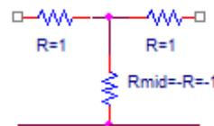
Figure 2: A negative impedance converter
