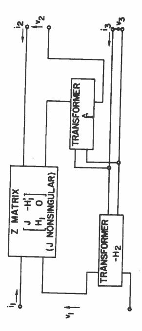
Figure 3. Hybrid Matrix Realization
