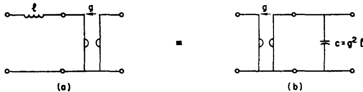
FIG. 2. Useful gyrator equivalence.
