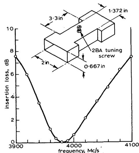
Fig. 2 Performance of one T section filter
