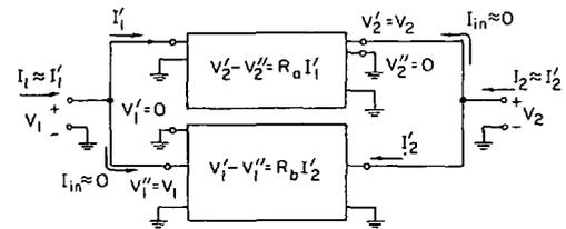
Fig. 1 Gyrator as differential voltage/current converters
