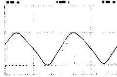
Fig. 7 Neural Oscillator Output. Oscillating Frequency 19.6 MHz.
