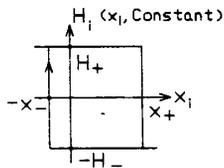
Fig. 2 Hysteresis Loop Characteristics of a Neuron Model.
