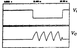
Fig. 8  $V_C$  shown in the Upper Trace, and  $V_N$  in the Lower Trace. For an Oscillating Frequency of 92.0028 KHz.
