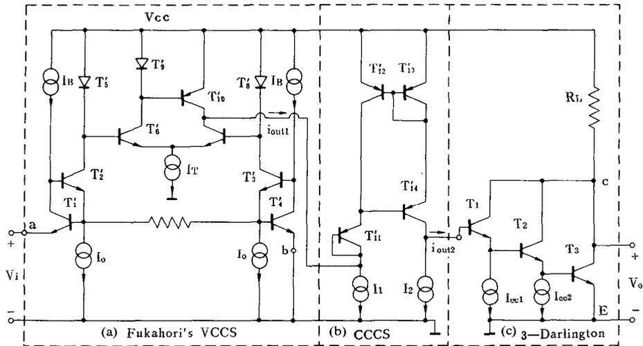
Fig. 2. Circuit and sections of integrator. (a) Fukahori's VCCS. (b) One scheme of CCCS. (c) 3-Darlington stage.
