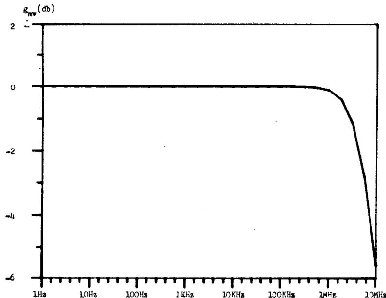
Fig. 6. Frequency response of the input VCCS.
