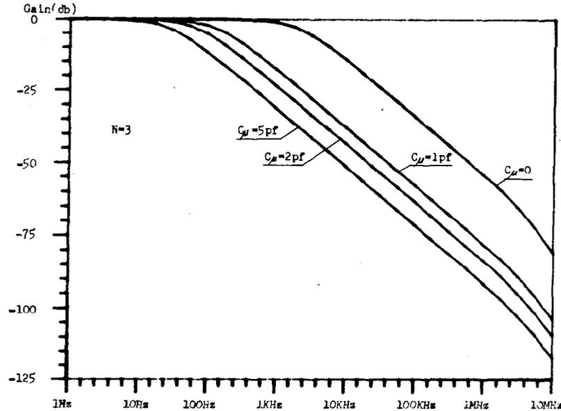
Fig. 5. Frequency response of integrator with different  $C_\mu$  under  $N = 3$ .
