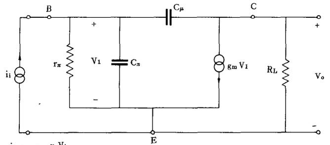
Fig. 3. Equivalent circuit of  $N$ -Darlington stage.
