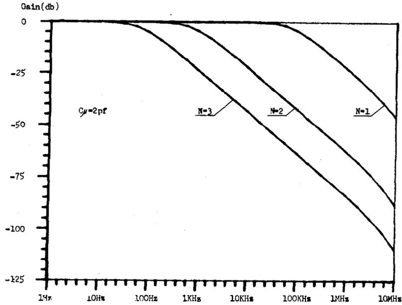
Fig. 4. Frequency responses of integrator with different  $N$  under  $C_\mu = 2$  pF.
