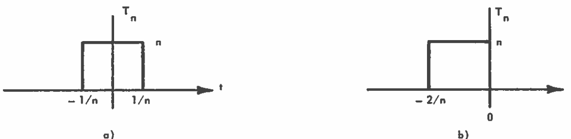
FIG. II-3. SEQUENCES OF DISTRIBUTION CONVERGING TO 2\delta .
