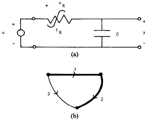
Fig. 7. (a) Circuit with semistate but no state equations. (b) Graph.
