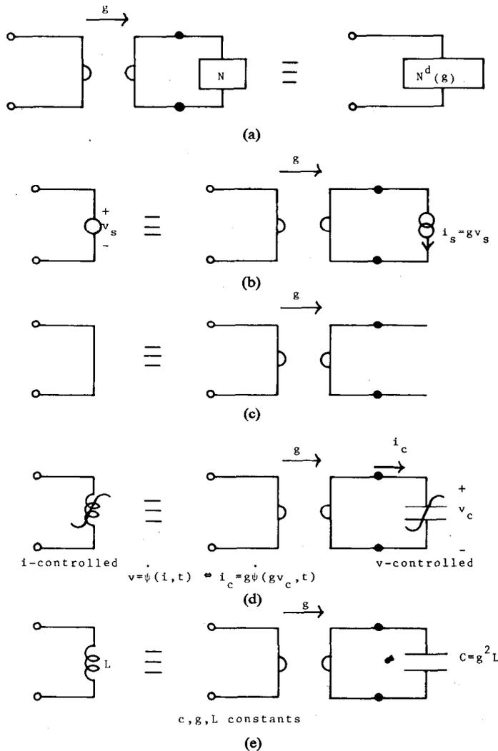
Fig. 2. (a) Basic one-port duality. Special Cases: (b) Voltage source replacement. (c) Short circuit replacement. (d) Current-controlled inductor replacement. (e) Time-invariant inductor replacement.
