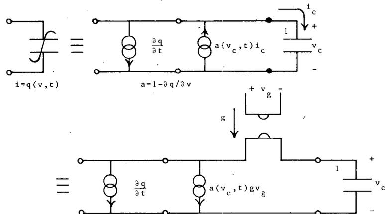
Fig. 4. Linear dynamics for nonlinear voltage-controlled capacitor.
