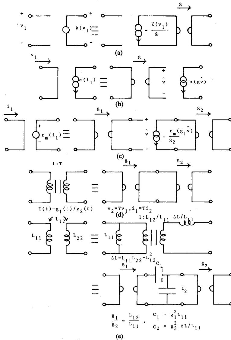
Fig. 3. Two-port equivalences. (a) VCVS. (b) CCCS. (c) CCVS. (d) Ideal linear transformer. (e) Time-invariant linear coupled coils.
