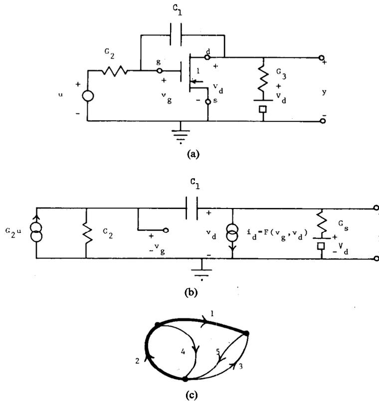
Fig. 6. (a) MOS example circuit with (b) equivalent and (c) graph.
