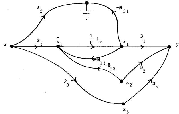
Fig. 9. Signal-flow graph for canonical linear time-invariant semistate equations.
