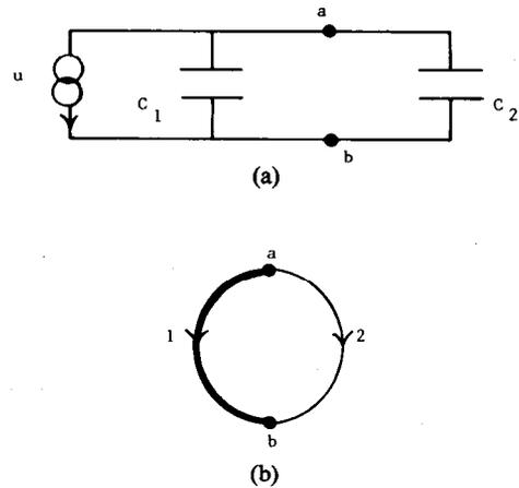
Fig. 8. Capacitive loop example circuit.
