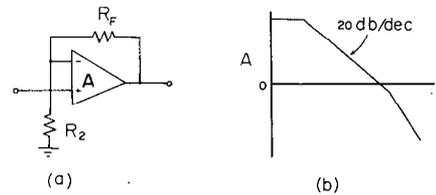
Fig. 1. (a) Noninverting op-amp stage. (b) Open-loop frequency response.
