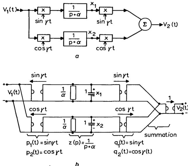
Fig. 2 Degree-2 time-invariant 2-path filter
