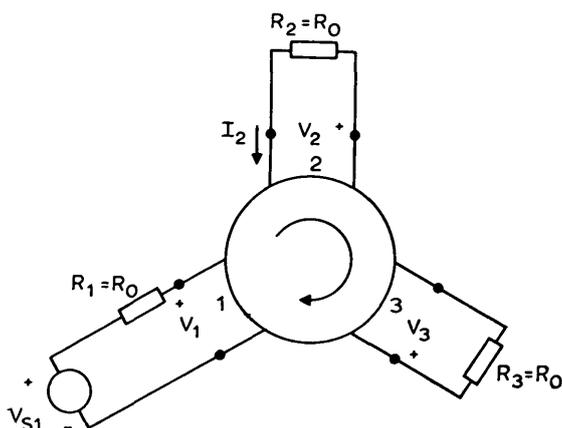
Fig. 1A Ideal lossless 3-port circulator
