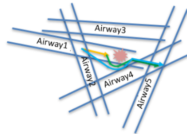
Fig. 4. Collision avoidance operation deviates the UAV from its original airway and might have effects on the air corridors of other aircraft (schematic is not drawn to scale, especially in airspace)
