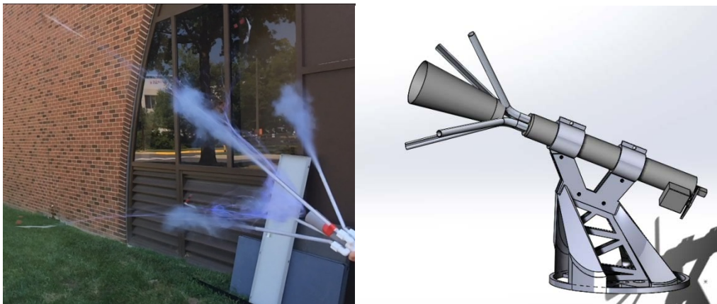
Figure 10. Net Launcher Design. Left panel: A snapshot of a net launch. The left-side corner weights can be seen at the left edge of the photo. Right panel: CAD drawing of the net launcher. The 4 corner-weight launch tubes and the central net cup can be seen. The main tube contains the CO 2 cartridge spring and seal-puncture pin. The spring is released by a servo motor controlled by the Raspberry Pi 2.0 computer. The launcher is constructed from four polycarbonate tubes, one central aluminum tube and 3D printed parts.
