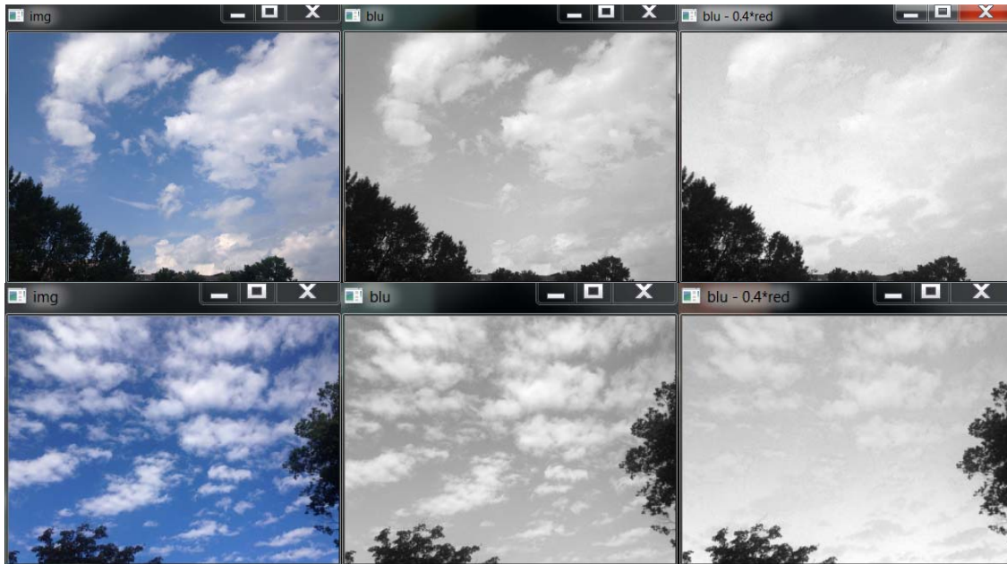
Figure 4. Further reduction of contrast for bright clouds. Two example images (rows): Left column: original color image; middle column: blue channel alone; right column: blue - 0.4*red. Due to the overall reduction in intensity from this operation, an intensity normalization is also performed.
