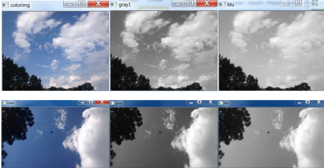
Figure 3. Reduction of the contrast of clouds by utilizing only the blue channel in an RGB image. The left column shows the original color image, the middle column shows a conversion to grayscale and the right column shows the blue channel image.
