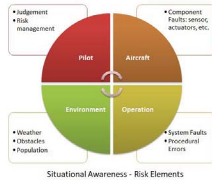
Figure 1. Fundamental risk elements for situational awareness: core elements which affect flight safety at all stages of flight.
