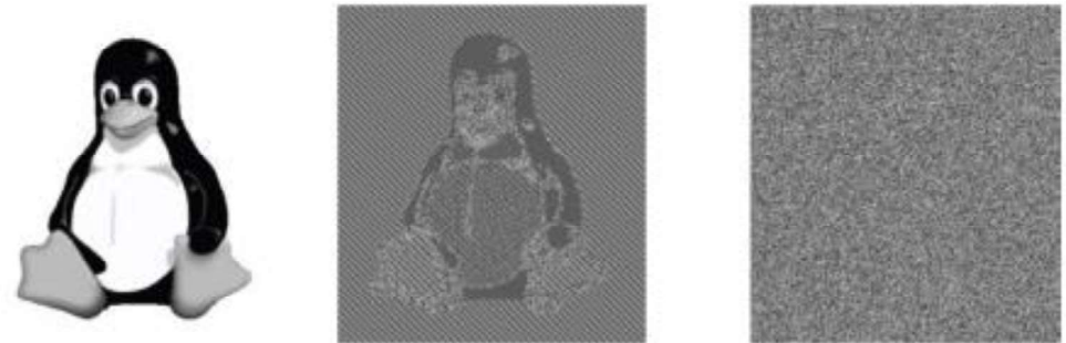
FIGURE 3.6: An illustration of the dangers of using ECB mode. The middle figure is an encryption of the image on the left using ECB mode; the figure on the right is an encryption of the same image using a secure mode.
