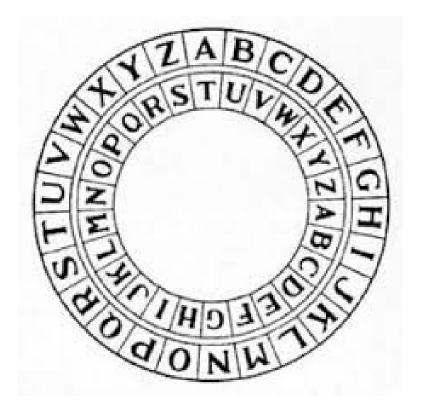
Example: Caesar cipher with shift 19.Outer wheel is plaintext letter.Inner wheel is ciphertext letter.
