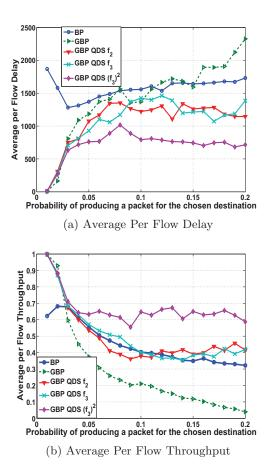
Figure 5: GRID Topology - Long Range Communication Scenario.
