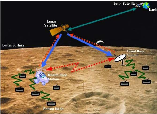
Figure 1. Proposed sensor network on remote planetary surface
