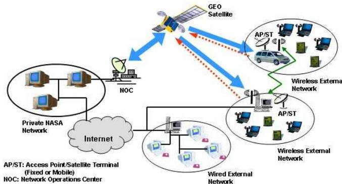
Figure 3. Interplanetary mission terrestrial network with GEO satellite
