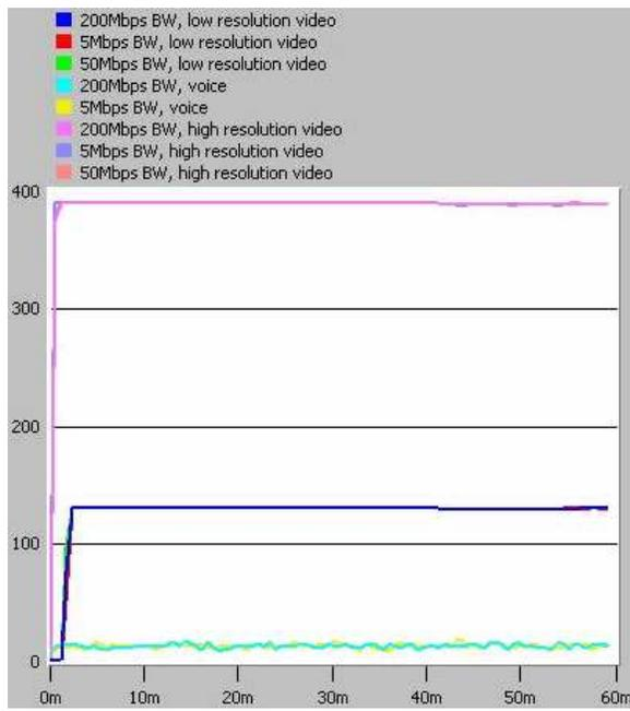
Figure 7. Satellite link throughput (packets/second)
