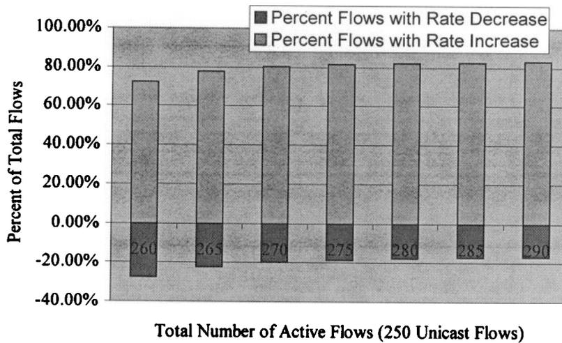
**Figure 5: Percentage of flows experiencing a rate increase or a rate decrease in their sustainable rates at the NOC for 250 unicast flows and 10 to 40 multicast flows under BAS-I policy with respect to the sustainable flow rates under EAS policy.**
