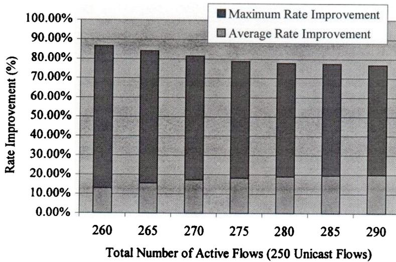
**Figure 6: Maximum and average percent improvement experienced by the sustainable rates of active flows at the NOC for 250 unicast flows and 10 to 40 multicast flows under BAS-II policy with respect to the sustainable flow rates under EAS policy.**
