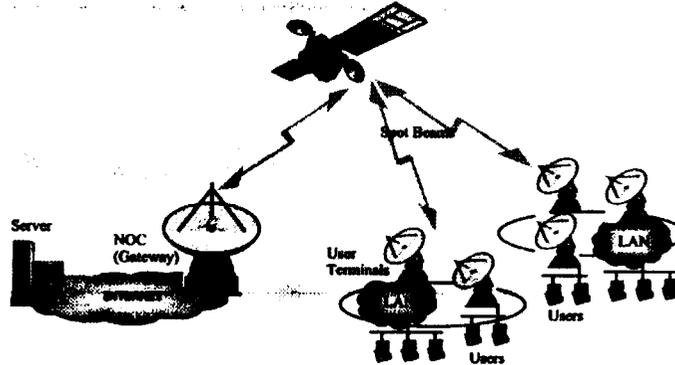
Figure 1: Satellite Network Architecture
