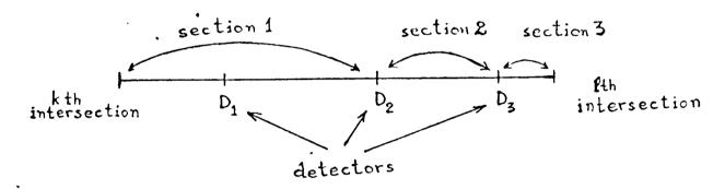
Figure 1. Illustrating the sections of a link of the network.
