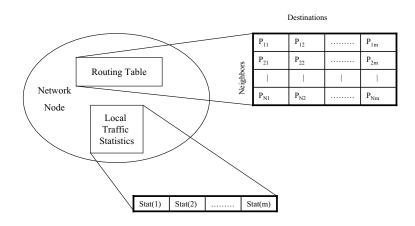
Figure 5.1: The routing table and local statistics table maintained at each node.
