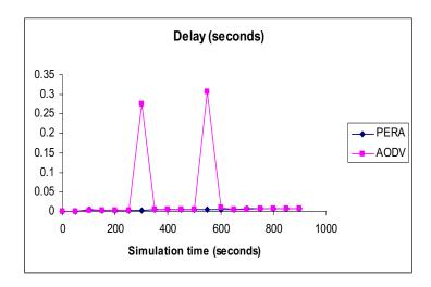
Figure 7.9: A delay comparison of AODV and PERA at 1 m/s.
