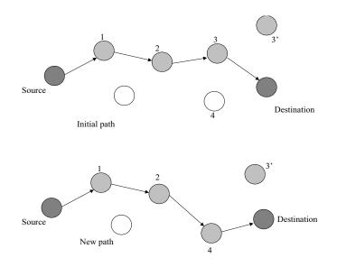
Figure 5.7: A new path is found by using probability adjustments in the case of link breakage due to node movement.
