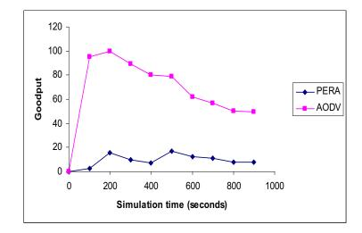
Figure 4.2: Goodput comparison of AODV and the unicast swarm based algorithm for 20 nodes in an area of 500m X 500m for speed of 1 m/s.
