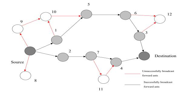
Figure 5.3: Each broadcast forward ant generates multiple forward ants and may find multiple paths to the destination.
