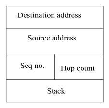
Figure 5.2: The structure of forward and backward ant packets
