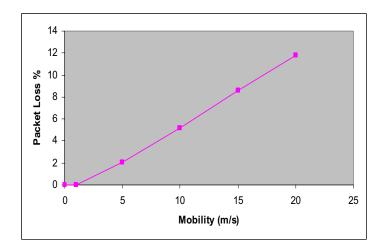
Figure 7.2: The percentage packet loss for varying mobility with 20 nodes in 500m X 500m.
