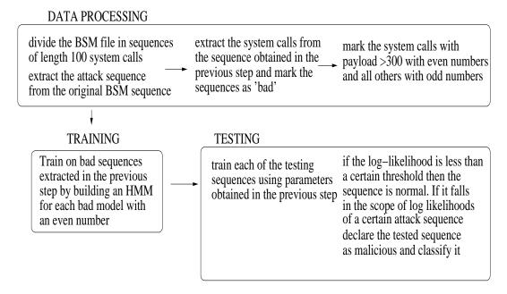
Figure 4.3: Detection and classification system scheme.
