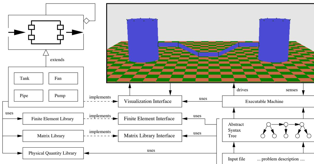
Figure 4. Architecture for modeling HVAC systems as networks of connected components, and using finite element solution procedures for computing and visualizing time-history behavior.
