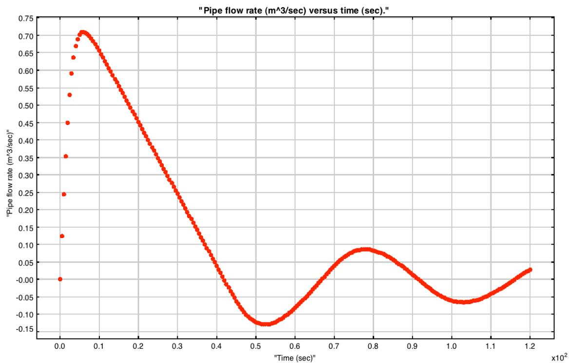
Figure 14. Volumetric flow rate ( $\text{m}^3/\text{sec}$ ) versus time (sec).
