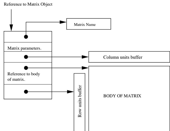
Figure 7. Layout of memory in matrix data structure.
