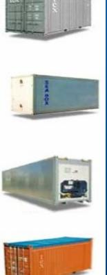
Dry Freight Container - used for goods that are not affected by most weather conditions such as clothing, automobiles, etc.
