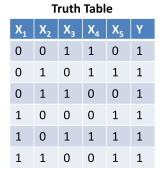
Truth table shows all input combinations for which output is 1
