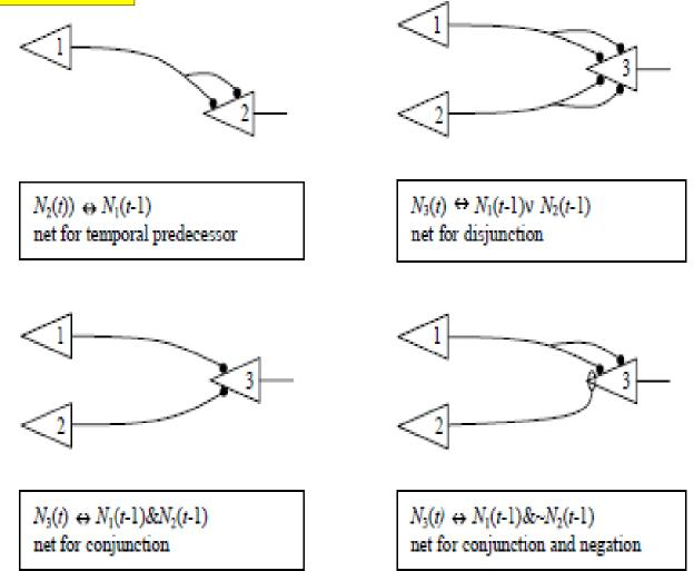
Figure 1. Diagrams of McCulloch and Pitts nets. In order to send an output pulse, each neuron must receive two excitory inputs and no inhibitory inputs. Lines ending in a dot represent excitatory connections; lines ending in a hoop represent inhibitory connections.
