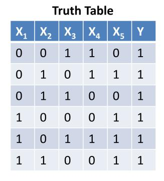
Truth table shows all input combinations for which output is 1
