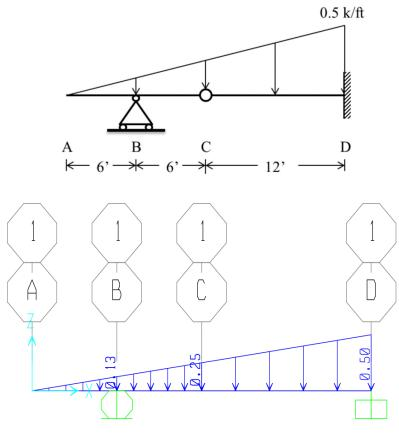
Reactions:  $R_B = 1 \text{ kips}$ ,  $R_D = 5 \text{ kips}$
