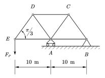
Use method of superposition for this linear elastic structure and assume  $F_P = 1 \ kips$ , the vertical reaction forces at A and B are:
