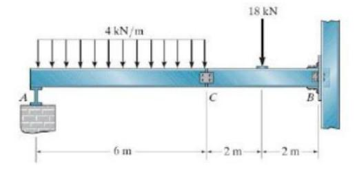
3) Determine if structure is stable or unstable. If stable, find out if determinate or indeterminate. Also find degree of indeterminacy id applicable. (10 points)
