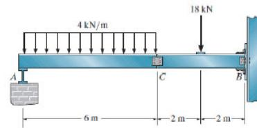
**Equations of Equilibrium:** First consider the FBD of segment AC in Fig. a.  $N_A$  and  $C_y$  can be determined directly by writing the moment equations of equilibrium about C and A respectively.
