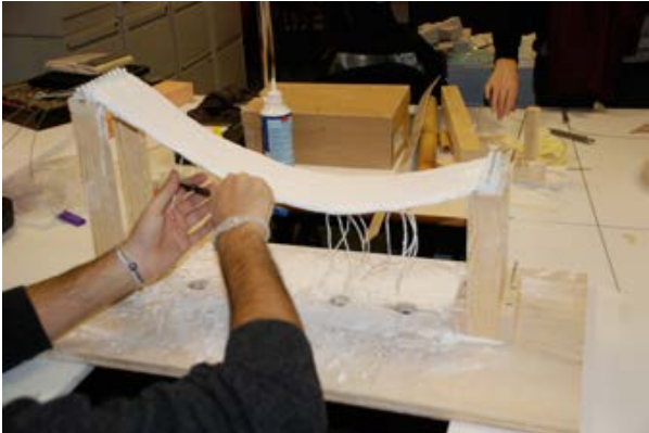
Using plaster and Plaster Hardener applied over 2 layers, making sure to cover the wire and cloth equally from both directions.
