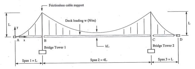
Figure 6: Elevation view of a three-span suspension bridge.
