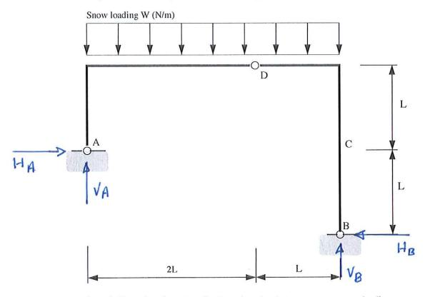
Figure 3: Front elevation view of a three-pinned arch that supports a snow loading.
