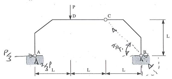
Figure 3: Front elevation view of a simple three-pinned arch.
