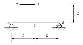
Assuming EI is constant for the structure and EA is sufficient large.
