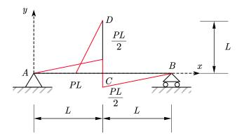
Bending Moment Diagram (virtual load):
