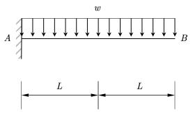
Use the *method of moment-area* to calculate the vertical displacement at point B, assuming the EI is constant along the beam.
