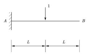
(1) Use the *method of moment-area* to calculate the vertical displacement at point B, assuming the EI is constant along the beam.
