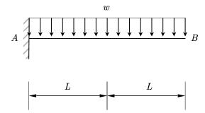
Use the *method of moment-area* to calculate the vertical displacement at point B, assuming the EI is constant along the beam.
