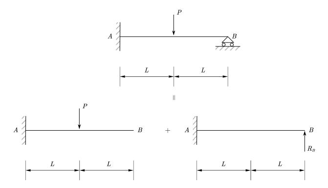
For the first beam, we can use the principle of superposition based on the solution in (1). Now, we are dealing with the second one:
