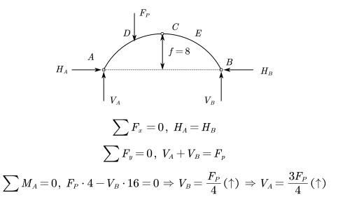
Slice the arc structure at point C, and write the moment equilibrium about point C (left part) would get:
