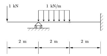
(1) Determine the structure as statically determinate, indeterminate or unstable. If it is statically determinate, point out stable or not; if it is statically indeterminate, point out the degree of indeterminacy.
