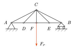
**Problem 2:** If the maximum force that any member can support is 10 kips in tension and 7 kips in compression, determine the maximum force  $F_P$  can be applied on the following structure (all the angles are  $\pi/3$ ).
