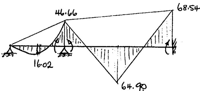
Determine the distribution of bending moments induced in the two-span beam when joint 3 settles by 30 mm. EI is constant along the full length of the beam.
