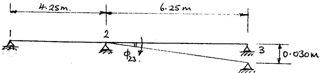
The chord rotation  $\phi_{23}$  is clockwise and positive, so the term  $(\frac{3u}{L})$  is negative. The F.E.M. are all zero - no applied loads.
