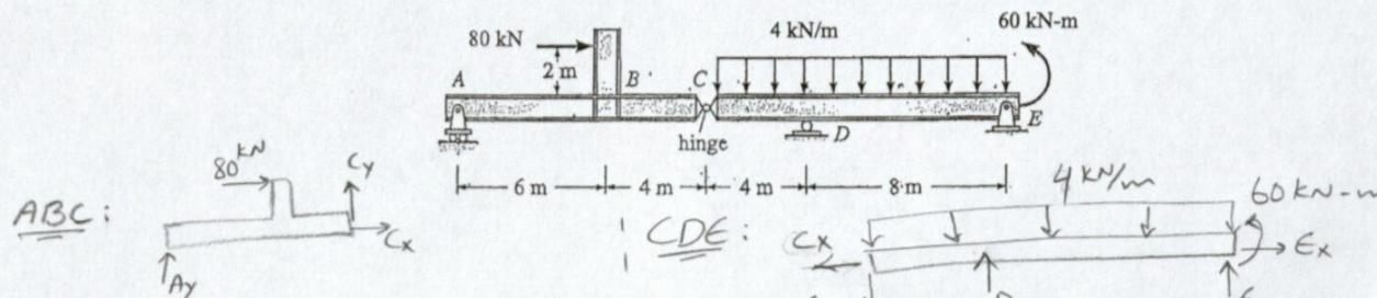
$$\begin{aligned} \text{ABC: } & \sum F_x = 0 \Rightarrow 80 + C_n = 0 \\ & \Rightarrow C_n = -80 \text{ kN} \end{aligned}$$
