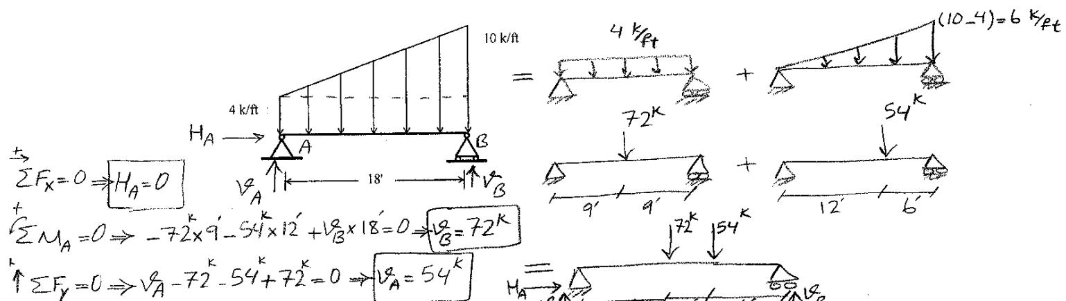
3. Classify the structure as statically determinate, statically indeterminate, or unstable
