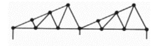
saw-tooth truss skylight
