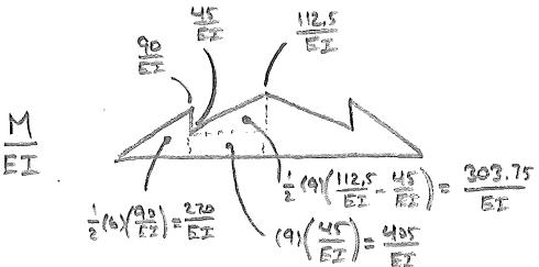
$$y_c = t_{A/c} = \int_A^C \frac{M}{EI} dx = \frac{270}{EI} (4) + \frac{303.75}{EI} (6+6) + \frac{405}{EI} (6+4.5) = \frac{8977.5}{EI}$$
