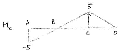
$$M_c \text{ due to load at A} \\ \text{At } C: \sum M_c = 0: 1(20) - 1.5(10) + M_c = 0 \\ \Rightarrow M_c = -5$$
