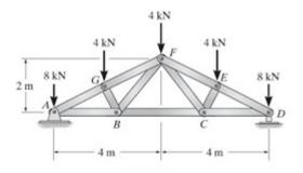
**P3** Determine the force in members *GF*, *FC*, and *CD* of the bridge truss. State if the members are in tension or compression. Assume all members are pin connected.
