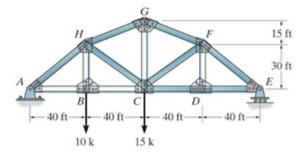
**P4** Determine the force in members *IH*, *ID*, and *CD* of the truss. State if the members are in tension or compression. Assume all members are pin connected.
