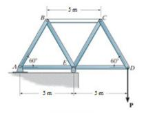
**P2** Determine the force in each member of the truss. State if the members are in tension or compression. Assume all members are pin connected. AG = GF = FE = ED.
